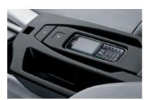
☐ Business preparation for mobile telephone with Bluetooth interface (with hands-free system, connection for recharging and external aerial). A separately available snap-in adapter enables connection of a Bluetooth-compatible mobile phone, which can also be operated via the iDrive Controller (in conjunction with navigation system\*). For mobile phone options contact your BMW partner.
