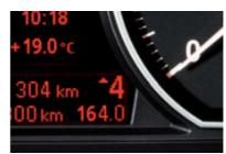
■ Shift Point Display for vehicles with 6-speed manual transmission shows when switching to another gear would be more fuelefficient; the system recommends when to switch to a higher or lower gear.
