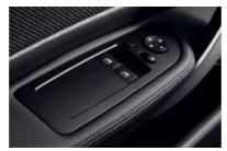
■ Window lifts, electric pull/press switch and "open/close" fingertip control, all-round comfort closing function and trap release.
