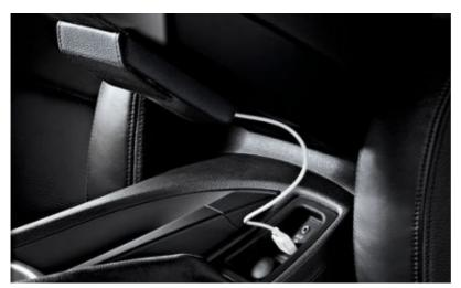
■ AUX-IN connection incl. 12-V socket for an external audio source such as a MP3 player. ☐ USB/audio interface for connection of a USB stick or MP3 player. Stored tracks are shown on the display of the Radio Professional (optional) or on the control display included in a navigation system\* option. Tracks are selected using the buttons on the optionally available multifunction steering wheel, Professional radio iDrive controller. A multimedia bag is supplied along with the optional armrest.
