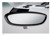
□ Interior mirror, with automatic anti-glare function and large surface area; the glare from following vehicles is automatically reduced when the amount of incident light exceeds a defined limit.
