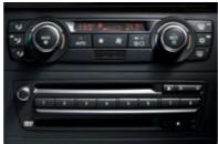
☐ Automatic air conditioning (shown here), with AAR, microfilter, fogging and solar sensors and residual heat button, quickly establishes and maintains the selected temperature. With separate temperature control for left and right sides.
