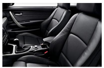
☐ Sport seats for driver and front passenger (shown here with optionally available Boston leather upholstery in Black), with infinitely variable electric backrest width adjustment for optimum lateral support, plus manual adjustment of fore-and-aft position, seat height, backrest angle, seat angle and thigh support (standard on 135i).
