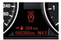
■ Auto Start/Stop display signals on the info display when the engine has been switched off by the Auto Start/Stop function (e.g. at traffic lights or in a jam). The engine is re-started automatically when you next press the clutch, and the signal is turned off (for the 120d and 123d in conjunction with a 6-speed manual transmission).
