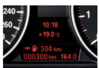
■ On-board computer, provides information about average speed, average and current consumption, radius and outside temperature. Also features an acoustic ice warning system.
