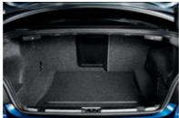
■ Luggage compartment, illuminated and with all-round textile lining; safe transportation is ensured by an elastic strap on the left-hand side, a flexible storage net on the right and lashing points on the inside edge. (Pictured is the optional storage compartment package).
