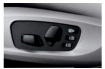
☐ Seat adjustment for driver and front passenger with electric seat height and backrest adjustment, as well as fore/aft and seat angle adjustment, with memory function for driver's seat and exterior mirrors (including automatic kerb focus). Two personalised positions can be stored for the settings of the driver's seat and the exterior mirrors.
