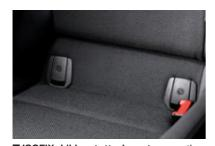
■ ISOFIX child seat attachment, rear on the two outer rear seats for safe attachment of a child seat with clip-in plug connectors plus additional fastening points on the upper part. □ ISOFIX child seat attachment for passenger seat. Passenger airbag can be deactivated per key.
