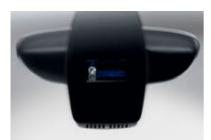
□ Rain sensor including automatic driving lights control: Once activated, the rain sensor will automatically switch on the windscreen wipers when it begins to rain, adjusting the wiper frequency in line with rainfall intensity. The integrated automatic driving lights control activates the low beam automatically at dusk and in tunnels.
