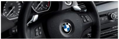
□ Paddles on steering wheel (in conjunction with 6-speed automatic transmission) for manual gear changing without using the clutch (planned availability as of March 2008).
