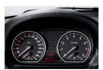
■ Dashboard: the 135i features special scaling with extra display ranges.
