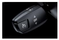
□ Cruise control stores and maintains a desired speed above approx. 30 km/h (activated using the left-hand steering-column stalk). After accelerating, the vehicle automatically returns to the previously stored speed. Braking cancels the setting.
