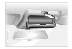
Press the button to open; fold upward to close.
