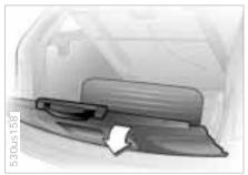
5 Press the tailgate down and hold it there. The spare wheel is now pulled by means of the removal aid onto the tailgate.
