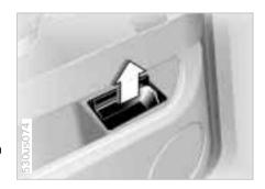
**To open**Rotate the cover upward.
