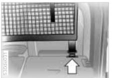
7 When the seatbacks are folded over, you can open the Velcro strips, completely unroll the partition net, insert it in the front brackets on the roof and attach the three hooks into the eyes. The illustration shows securing at the bottom right as an example.
