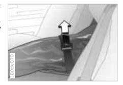
Secure the bag's contents by tightening down the retaining strap at the buckle.
