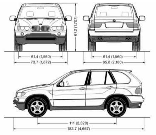
All dimensions are given in inches (mm). Min. turning circle dia.: 39.7 ft (12.1 meters)
