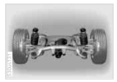
This axle is based on the same multilink principle as that in series-7 vehicles. The axle's kinematics and elastic kinematics are critical for wheel control - a significant prerequisite for achieving the objective of exceptional onroad handling characteristics with this vehicle concept.
