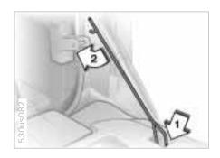
6 Insert support rod in tailgate lock and press down until it engages (arrow 1); then lock hook of rod in striker (arrow 2).
