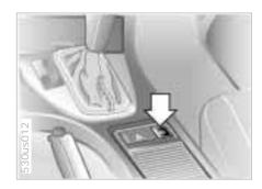
You can operate the central locking system with this button (arrow) when the driver's door is closed. The doors and liftgate are unlocked or locked only. However, the antitheft alarm system is not activated. Also, the fuel filler door remains unlocked to allow refueling.
