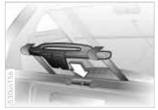
3 Hook both buckles into the latch of the tailgate (arrow); the tailgate is released.
