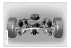
The level control system for the rear axle maintains constant ground clearance of your vehicle, even when carrying a load.
