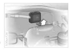
4 Start by connecting the jumper cable from the positive terminal of the support vehicle to the positive terminal connector located in your BMW's engine compartment The cover of the auxiliary terminal for jump starting is marked with a "+" sign (refer to the illustration). To remove the cover, tip up the cap (arrow).
