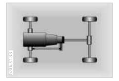
The transmission of power to the four drive wheels is provided permanently through a transfer box. The distribution of torque between the front and rear axles is 38 % to 62 %.
