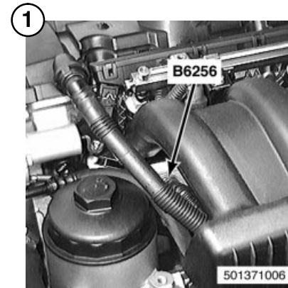
B6256 DUAL TEMPERATURE SENSOR (COOLANT TEMPERATURE)
