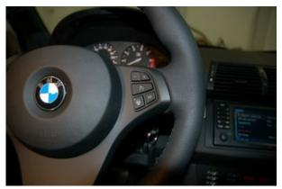
Reconnect the battery at this point and turn the ignition to the on position. Press the heat button on the steering wheel and it should light up.
