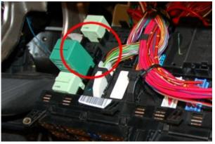
On the left side you should see an empty spot for a relay. This is where your new relay should fit for the heated steering wheel. Simply push the relay into place – it only fits one way so you can't put it in the wrong way.
