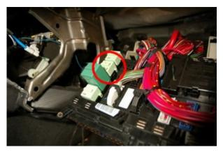
Here is a pic with the relay installed. Re-install the fusepanel into it's place.
