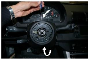
Remove the small screw on the top of the steering column as shown using a Phillips screwdriver. Once you remove the screw, there is also a small black plastic anchor piece that needs to be removed. Use a small flat head screwdriver to pry it out.
