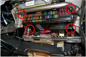
With the glovebox out of the way you should have access to the fusepanel.
