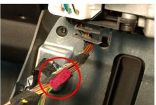
If your car is pre-wired for the heated steering wheel, you will see this small red connector taped back behind the steering column switch.
