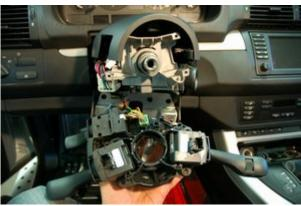
The column switch should come off easily. Remove all wiring connectors from the back of the switch. Take the steering column switch off completely.
