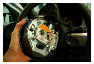
Reinstall the airbag connectors to the airbag that goes with this steering wheel.
