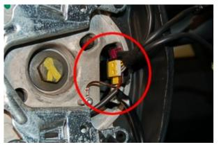
Reconnect the airbag connectors and new red connector for the heated steering wheel as shown.
