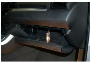
Open the glove box and disconnect the light. The light should be on the inner side close to the latch and should easily snap out. There are no screws in place.
