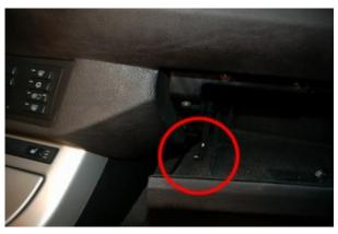
On the left side there is a plastic arm that slides down. Lift the glove box just a touch and remove the plastic rivet holding it in place. This should just slide out to the left.
