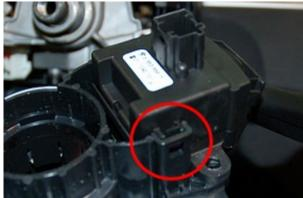
Next remove the indicator stalk and the wiper stalk. These simply snap into the column switch.
