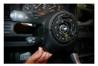
Screw the new column switch into place.
