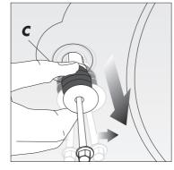
Remove transport safety bolts and rubber bushes by pulling outwards. (A up/down action and a small squirt of washing up liquid should ease removal.)
