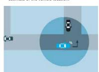
2. After just a few metres, the road the vehicle is travelling on can be identified. Any turns are recorded by the gyroscope.
