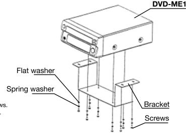
**1.** Fix the pracket to the unit with screws.
