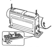
Remove the hexagonal nuts and take off the changer.
