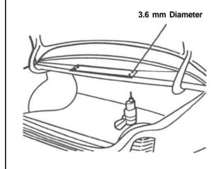
• Attach the CD changer with the tapping screws (M5 x 12).
