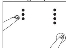
To start a new program after the program is over or to interrupt the program, the childproof lock should be deactivated. To deactivate the childproof lock, press the same buttons for 2 sec. The "Childproof lock" will be deactivated and the warning light will go off.
