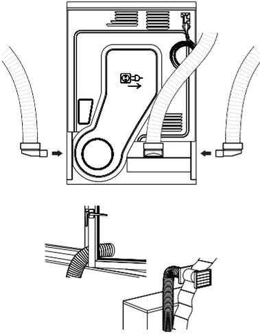
water out through the water drain hose supplied with the machine instead of periodically draining the water collected in the water tank.
