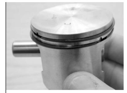
13.18 Align piston in correct orientation.
