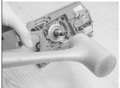
20.8 Remove the bearing from the flywheel side of crankshaft.
