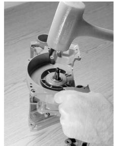
20.5 Remove the flywheel side crankcase seal with 1/2" (13 mm) socket.
