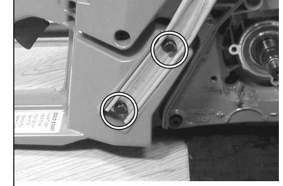
18.2 Remove front handle screws on bottom.
