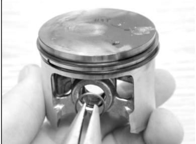
13.16 Make sure wrist pin retaining clip is in the proper orientation.
