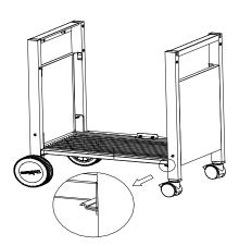
**Step 3** Unfold cart frame, as shown.
