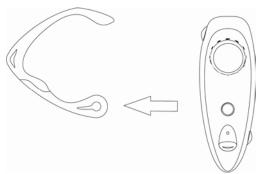
For left ear, simply unsnap the ear clamp from the headset by pulling gently at the case of the ear clamp ring.
