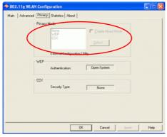
Privacy Mode | Configure your NONE \ WEP or CCX settings: NONE: No security defined. | WEP (Wired Equivalent Privacy) is a data security mechanism based on a 40 Bit/128 Bit/256 Bit shared key algorithm. Press the Select button to change WEP configuration. A new dialog window will be opened(see page 26)
