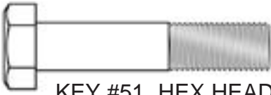
KEY #51 HEX HEAD BOLT 3/8" X 1 3/4" PARTIAL THREAD QTY. 10
