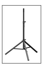
5. To lower speaker, remove the safety pin from the slot. Slowly loosen the hand knob. Use caution and slowly lower the upper telescoping tube. Tighten hand knob and remove speaker cabinet.
