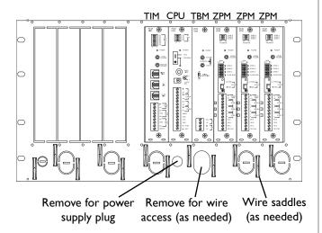
A 15-zone PCM system without talk-back capability, six-zone slave assembly mounted at left:
