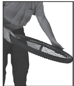
Figure 6- On an angle, rotate the wheel to distribute the sealant
