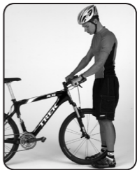
Figure 1- Function testing the handlebar and stem
