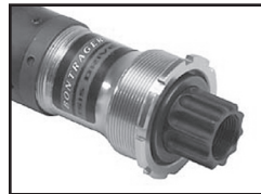
Figure 5- Splined bottom bracket axle
