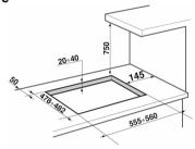
Make sure there is a minimum of **750 mm** between the hot plate flames and any shelf that may be installed directly above them.
