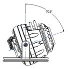
Figure 4.4 Maximum tilt angle of 70 degrees
