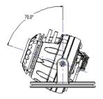
Figure 4.5 Maximum tilt angle of 70 degrees
