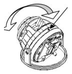
Figure 4.2 Tilt adjustment
