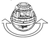
Figure 4.1 Pan adjustment
