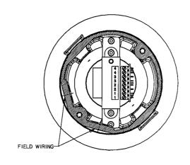
Numbers on Terminal Label are in pairs to facilitate loop-in loop-out option. Terminals are linked via PCB tracking.
