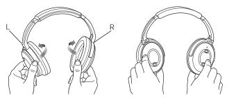
**Note:** Incorrectly rotating the earcups can damage the headphones.
