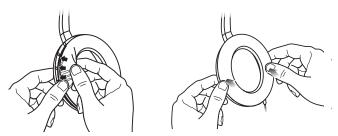
If an earcup cushion becomes partially or completely detached, push its mounting flange back into the earcup. Then use your finger or thumb to press around the edge of the mounting flange, making sure it snaps into place all the way around the earcup.
