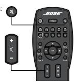
**Note:** Make sure the internal speakers in your TV are turned off. To confirm, press Mute on the Bose remote and check that no sound is coming from the TV. For more information, refer to "Turning off the internal speakers in your TV" in the Setup Guide.
