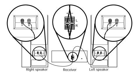
Unscrew the hex knobs on the terminal posts (Figure 5) located on the back of the left (L) speaker. This reveals a small opening through each post where the wire goes.
