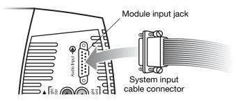
At the other end of the system input cable, multiple wire pairs "unzip" for easy reach and insertion into terminals on your receiver. A red collar marks a wire as positive (+) wire.
