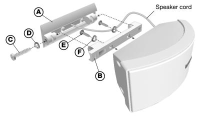
2. Hold bracket part **A** in position against the wall and mark the left and right round holes for the mounting hardware (Figure 4). If you plan to feed speaker cord through the wall, mark the oval speaker cord feed-through hole also.
