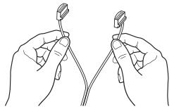
**3.** Plug the **LEFT** speaker cable into the rear jack of the left speaker (Figure 10). Plug the **RIGHT** speaker cable into the rear jack on the right speaker.
