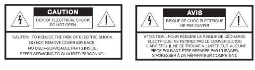
The lightning flash with arrowhead symbol within an equilateral triangle alerts the user to the presence of uninsulated dangerous voltage within the system enclosure that may be of sufficient magnitude to constitute a risk of electrical shock.
