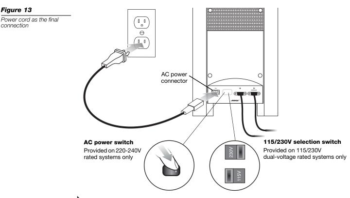
Note: On 220-240V models only, turn the Acoustimass® module POWER switch to on (I).
