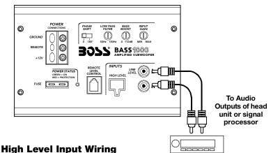
The high level input(s) should only be used when your receiver lacks RCA outputs. If the RCA outputs are not present, connect the speaker outputs from the receiver to the high level input connector of the amplifier. Be sure to observe polarity to
