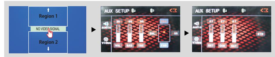
**Warning:** In AUX mode, you can adjust the angle of screen by press region 1 & region 2. Press Region 1 to slide up, press Region 2 to slide down.
