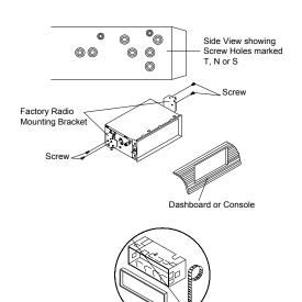
To fasten the unit to the factory radio mounting brackets.
