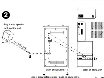
a) Connect the right front satellite's control cable (blue) to the "Control" jack (blue) on the back of the subwoofer.
