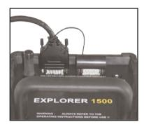
Once connected, switch the power on the Gemini(s) to position II. Switch the Explorer on. The Gemini(s) will now charge followed by the pack. Adjust the flash power on the Gemini(s) and set up as required. If more than one Gemini is fitted then wait until both are ready before firing. If the pack is being flashed simultaneously with the Gemini then the READY indicator on the pack indicates that the overall set-up is READY.
