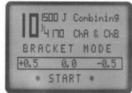
The unit will automatically check and warn if the selection is not possible within the existing setting constraints. A warning occurs if the bracket step will take the unit outside of its normal operating range.
