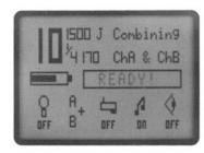
To set the flash power press the A or B button to select the required channel. The associated LED will light to show it is selected. Set the power for that channel by rotating the knob.
