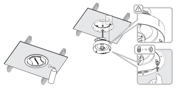
**4.5** If the frame flange is to be painted it should be done at this stage. Any conventional, domestic paint may be applied by brushing, rolling or spraying. Use the supplied paint mask to avoid getting paint in the cavity. Painting without using the paint mask risks contamination of the internal connection terminals or the grille attachment magnets. The diagram above illustrates painting using the paint mask.
