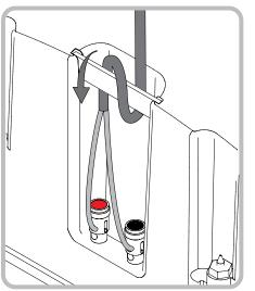
**4.4** Now connect the speaker cable to the spring terminals on the side of the back box, first looping the cable around the strain relief bar. A second person will be required to hold the back box while the cable is connected. The diagram above illustrates the cable connection.
