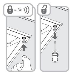
**4.8** The baffle can now be lifted up into the back box. Ensure that the connector on the baffle is oriented correctly with the connector inside the back box. The baffle is held in the back box by four pushlock fasteners. push-lock fasteners are secured by pushing the head inwards – either with a thumb or a screwdriver. As they secure, the fasteners will click.
