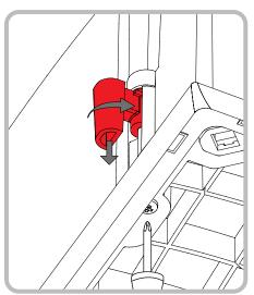
**4.5** With the back box connected it may be lifted up into the ceiling aperture. Correct back box orientation must be established at this stage: the red arrow on the back box flange should be pointing towards the listening area.
