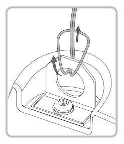
4.2 If speaker cable is already present in the ceiling space, pull the cable down through the aperture. If speaker cables are not already installed this should be done at this stage. It is likely that you will need to gain access through the floor above to route the cables through the ceiling space.
