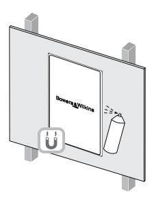
4.6 If the back box flange is to be painted it should be done at this stage. Any conventional, domestic paint may be applied by brushing, rolling or spraying. Use the supplied paint mask to avoid getting paint in the back box cavity. Painting without using the paint mask risks contamination of the internal connection terminals or the grille attachment magnets. The diagram above illustrates painting using the paint mask.
