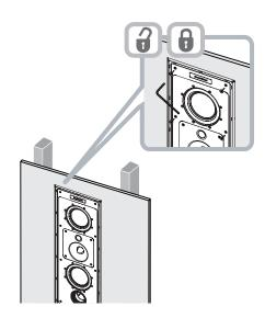
With the MF/HF baffle in the correct orientation the baffle assembly can be lifted and inserted in the back box till it is just sub-flush of the back-box flange. Take care to ensure that the electrical connector lines up. The baffle is held in the back box by eight screws. Tighten the screws to a torque of 1.5Nm. The baffle will then be secured in the back box.
