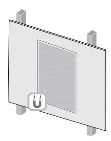
**4.9** The grille can now be fitted to the baffle. It is held in place magnetically so simply needs to be aligned with the groove in the back box flange where it will click into place. The diagram above illustrates fitting the grille.
