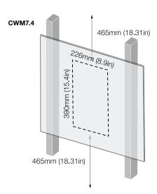
CWM7 Series in-wall speakers comprise a baffle carrying the speaker drivers and crossover, an integrated back-box and front flange, and a magnetically secured grille. The back box is connected via external terminals to the speaker cables with the baffle connecting automatically as it is inserted in the back box.
