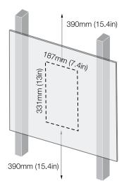
All CWM7 Series speakers require a clear depth of 102mm (4.02 in) from the front of the ceiling surface.
