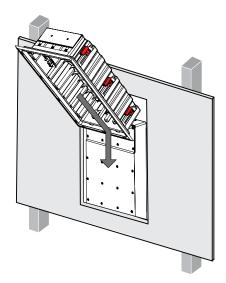
4.5 With the back box connected to the cable and its reservoir box attached it may be inserted into the wall aperture and cavity. Correct back box orientation must be established at this stage: the red arrow on the back box flange should be pointing upwards.
