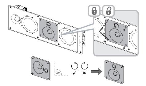
**4.7** The baffle can now be inserted into the back box. The baffle insertion and attachment technique is slightly different in the case of the CWM7.3 and CWM7.4/5. In both cases however you should first ensure that the connector on the baffle is oriented correctly with the connector inside the back box.
