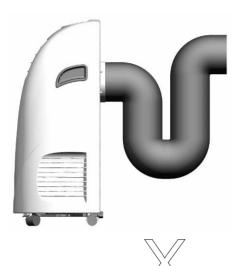
The bend of the exhaust pipe is very important. Incorrect mounting can prevent the machine from working correctly.
