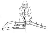
Use the plastic strap (attached to the last rung) to wrap and secure the rungs.
