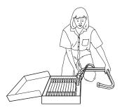
Lay the rungs, wrapped with the plastic wrap, in the box with the standoffs facing upward. Place the folded sill hooks on top of the rungs, between the standoffs.
