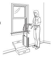
3. Place the sill hooks firmly over the windowsill and pull the release strap to deploy the ladder.
