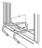
**DIMENSION A:** The windowsill width should be between a minimum of 6" (15 cm) and a maximum of 10" (25 cm).
