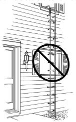
Do not use from a second floor window directly above a first floor window.
