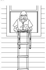
4. Exit carefully through the window and place your feet on the first rung. Hold onto the window frame until your weight is evenly distributed on the ladder. Climb down, keeping your body close to the ladder.
