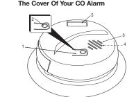
Test/Silence Button Scroll Button (CO5120PDBN) 2. POWER/ALARM Light (RED)
