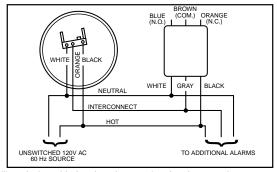
After installation, test the interaction of the auxiliary device with the alarm by pressing the alarm test button.
