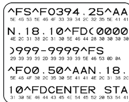
Figure 42 • Communications Diagnostics Test Label
