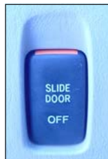
Switch OUT: Power Functions Enabled
