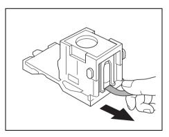
12 Insert the staple cartridge, making sure the tabs on the cartridge slide along the rails in the compartment.
