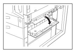
2 Turn the green wheels to feed the paper so that it can be easily removed.
