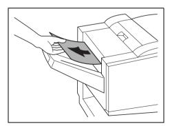
8 Open the transport guide, and then pull out any paper in the transport section.
