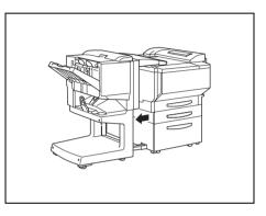
2 Pull out the hole-punch waste container.
