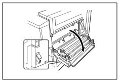
4 Turn the knob on the inside of the right-side door clockwise to feed out the paper.
