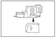
5 Insert the new staple cartridge into the staple holder, and then carefully pull out the stopper.
