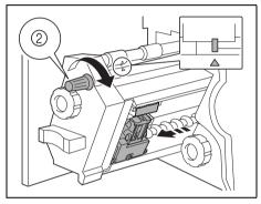
5 Grasp both sides of the staple cartridge, lift up the staple cartridge, and then pull it out.
