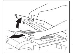
4 Open the feed guide for the finisher, and then remove any paper.
