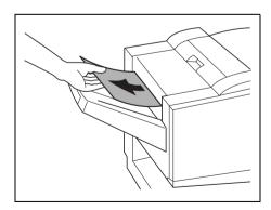
9 Open the feed guide for the finisher, and then remove any paper.
