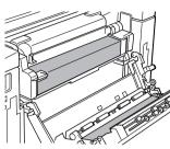
9 Grasp the tab on the left end of the fusing unit cover, and then swing the cover toward you to open it.
