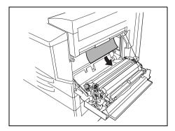
7 Grasp the upper right-side door as shown, and then carefully open the door completely while making sure to support it.
