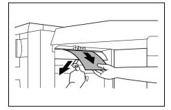
**10** Open the transport guide, and then pull out any paper in the transport section.
