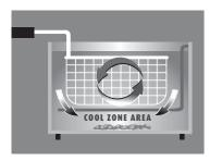
The submerged heating element system on the Avance Forte Deep Fryer allows oil to be heated more effectively, and respond quickly to oil temperature changes.
