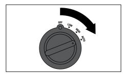
When cooking is complete, turn the Temperature Control Dial to the OFF position, switch off at the power outlet, remove the power plug and then the connector end from the appliance inlet.
