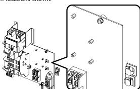
8. Install ACCM board into transfer switch using supplied screws in locations shown.
