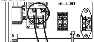
Slide one current transformer (CT) over each generator power supply lead and reconnect generator power supply leads to contactor terminals.
