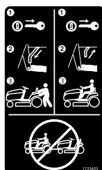
Decal - Transmission Release Part No. 1723425
