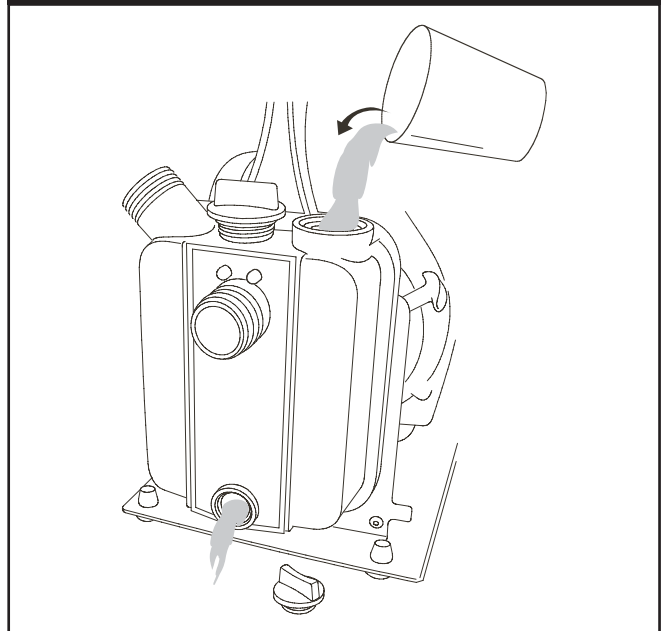
Figure 19 — Remove Plug from Top of Pump and Flush
