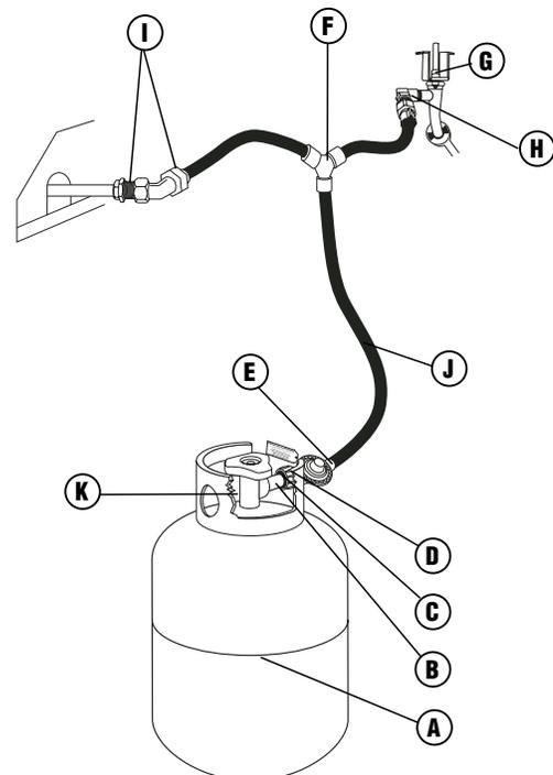
6. Check each place listed (A–K) for growing bubbles which indicates a leak.
