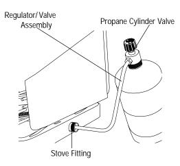
NOTE: Use propane cylinder upright when possible to prevent flare-ups. Make sure not to cross-thread fittings while tightening.
